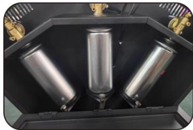
3. Align the nozzle of the spray oil bottle with the machine interface
