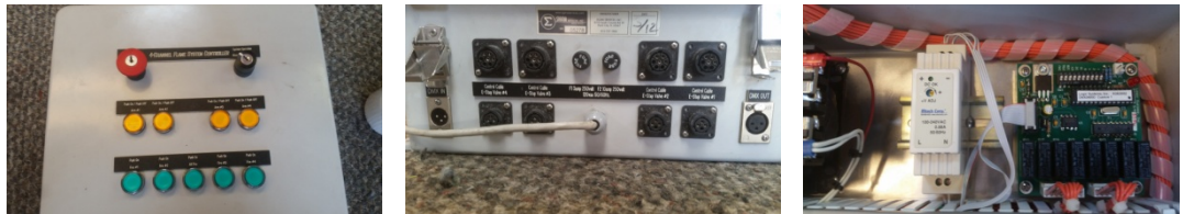
4- Channel Flame Control Panel – Manual Controls (Left), Cable Connections (Center), (DMX Relay Board (Right)
