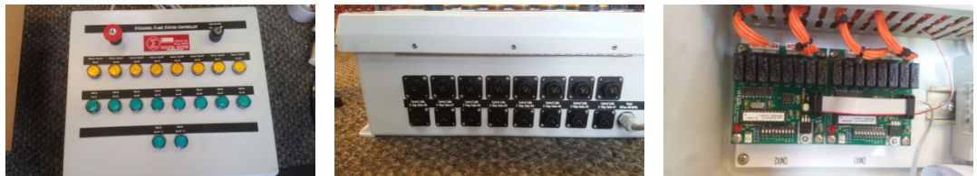
8- Channel Flame Control Panel – Manual Controls (Left), Cable Connections (Center), (DMX Relay Boards (Right)
