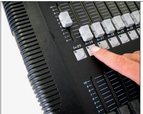
Press the flash button for the selected "fire" channel on the DMX controller. A flame should now be emitted from the Stage Flame.
