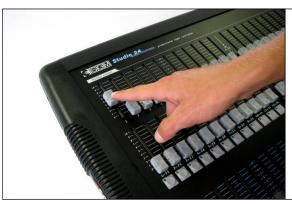
After you have used the Stage Flame, you must set it to safety mode again. You put the Stage Flame in safety mode by shutting the safety channel or setting it to a value outside the 40% to 60% range.
