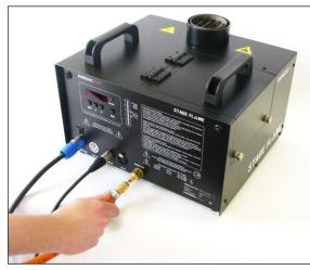
Attach the other quick release connector of the propane gas hose to the Stage Flame.
